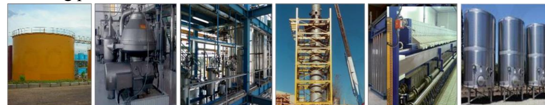
Crude Tank Degum Bleach Deodorization Fractionation Product Tank
